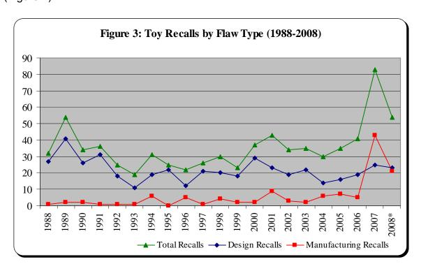
As presented in Figure 3, the number of toy recalls due to design flaws has always been higher than those due to manufacturing flaws, with the sole exception of 2007 when lead related recalls outnumbered the recalls due to design flaws. Since 1988, a total of
